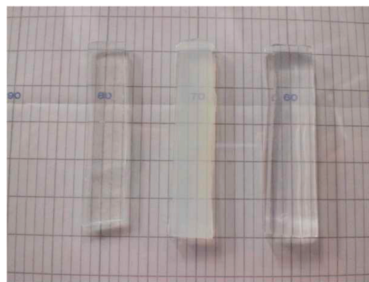
Figure 3. Appearance of the three types of polyrotaxane gels: (left) PRG/DMSO; (middle) PRG/W; (right) H-PRG/W. PRG/DMSO and H-PRG/W are transparent, while PRG/W is opaque.
